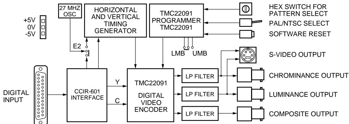
The board accepts 8-bit parallel digital component video, (CCIR Rec. 656 or SMPTE RP 125, a.k.a. "601") at a standard D25 connector in differential ECL format, translates the data to TTL format, strips the Timing Reference Signal from the datastream to generate H&V Sync, and passes the digital video stream to the Encoder in a 16-bit 13.5 MHz format.
